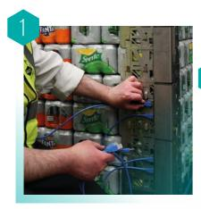
We mount electronic modules that measure the forces in 40 positions on each wrapped load, meaning we can identify over or under-use of wrap and too much force (which could lead to crushing) or too little force (which creates instability).
